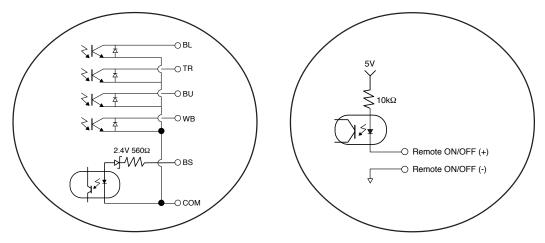
8. Example of the use of the Contact Signal circuit
